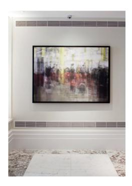
Linear wall diffusers for supply and extract air.
