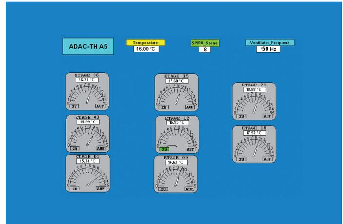
Fig. 6: Overview of the temperatures on the individual floors, outside temperature and setting of the damper motors for supply of air to the stairwell.
