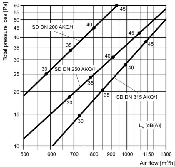
**Figure 3:** Sound power and pressure loss for SD AKQ/1 size 200, 250 and 315
