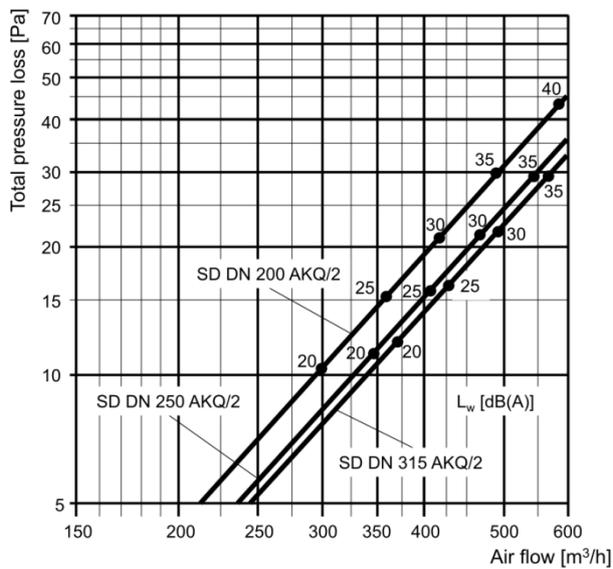
**Figure 3:** Sound power level and pressure loss for airflow of displacement section for diffuser sizes 200, 250 and 315
