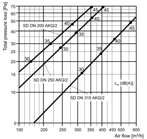
**Figure 3:** Sound power level and pressure loss for airflow of swirl diffuser for diffuser sizes 200, 250 and 315
