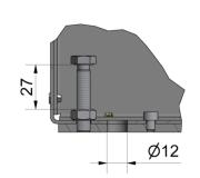
Screws for height adjustment to the floor
