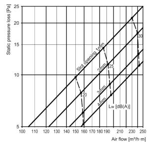
**Fig. 2:** Sound power level and pressure loss for linear floor diffuser in relation to air flow and damper position. Supply diffuser 200 rum wide, 1000 mm long. Air supply via two sides - slide plate with damper.
