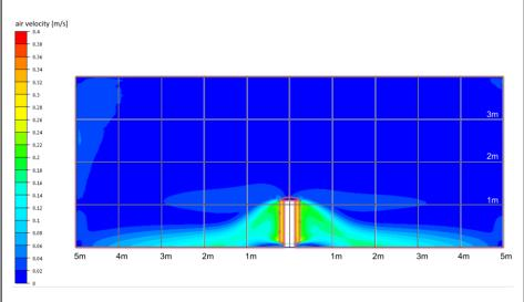
Fig. 2: Air velocity distribution with front velocity of 0,25 m/s and temperature difference room air to supply air of 3 K
