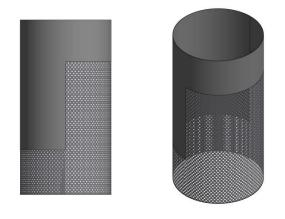
Using different sized perforated plates to form the inner cylinder provides different volume flows in each direction, again whilst all the units look the same.
