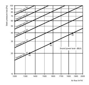
**Fig. 3:** Sound power level and pressure loss for binnacle diffuser NIQ-R 550/1000
