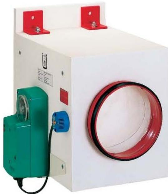
Before putting the ventilation systems into operation, all dampers shall be inspected on site. In the first year after putting the ventilation system into operation, the operational reliability test shall be carried out at least twice a year (from the central). If two consecutive tests show no malfunctions, then the functional test only has to be carried out once a year. Logging is necessary (DIN 13306).
