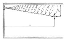
**Illustration 4** Illustration of horizontal and vertical depth of penetration
