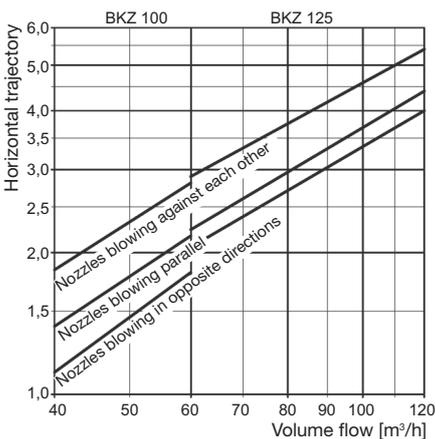
**Illustration 2** Horizontal trajectory length [m] depending on the volume flow
