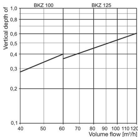
**Illustration 3** Vertical penetration depth [m] depending on the volume flow
