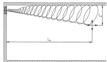
**Illustration 4** Illustration of horizontal and vertical depth of penetration
