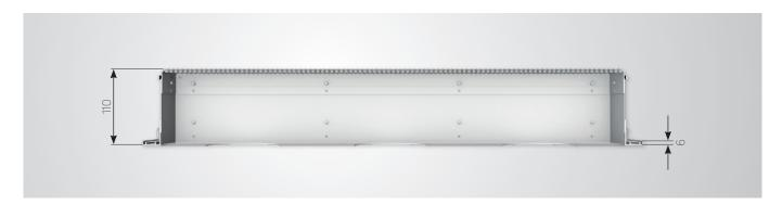
In order to achieve a uniformly designed room pattern, exhaust air variants of the WSA without swirl nozzles are available. Hole pattern of the front is optionally similar to that of the standard version or similar to the grille plate.
