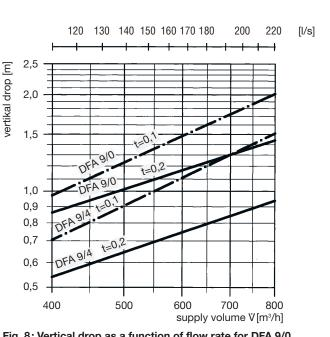
Fig. 8: Vertical drop as a function of flow rate for DFA 9/0 and 9/4.
