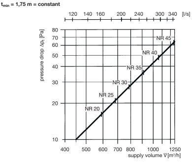
Fig. 12: Total pressure loss (Pa) and noise levels (NR) for Multi-outlet Swirl diffuser DFA-AKQ 9
