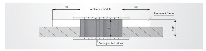
Classified installation shafts and ducts F90 - F120
