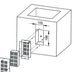
Maximum breakthrough dimension 105mm x 198mm. Installation frame is not mortared in. The intermediate space between installation frame and breakthrough is sealed by intumescent material.
