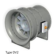
Туре DV2 Installation sizes 400 mm to 1,120 mm 0.75 to 45 kW Power range Repair switch, air-intake nozzle, Accessories, standard extension shaft, shaft feet Flexible connectors, counterflanges, protection grille, Accessories, optional diffuser, spring vibration damper, vertical brackets Axial fan with characteristic curve stabiliser, Short text impeller with adjustable blade and adjustable guide wheel Colour RAL 7030
