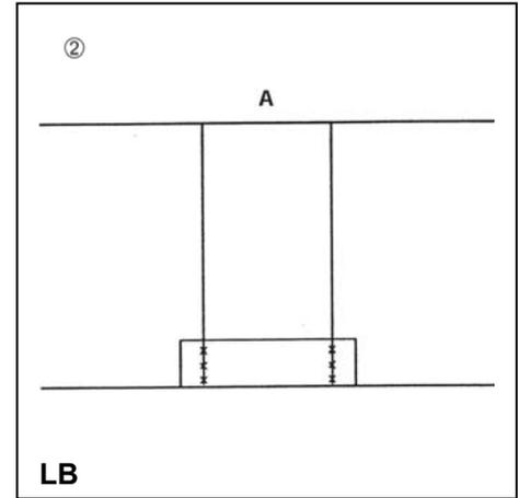
When dimensioning the hangers (slotted band), the load of 6 N/mm<sup>2</sup> shall not be exceeded.
