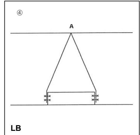
**A** = Steel dowels = M8 shall be used. They shall be inserted twice as deep as required by the test certificate – at least however 6 cm deep –, if the test certificate does not state otherwise. The calculated tensile load shall not exceed 500 N per dowel; compare DIN 4102 Part 4 (3/1981), clause 7.3 and 7.5.
