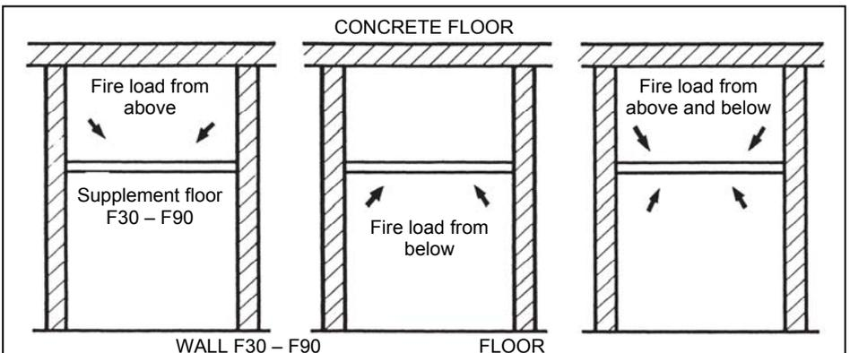
**Figure 2. Drawing of the different test requirements**
